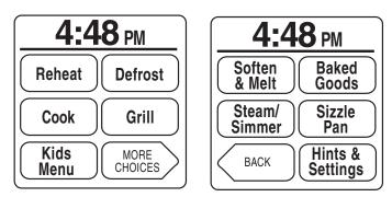
The LCD touch screen is used to input commands. A light- to medium-pressure touch of the fingertip will activate the menu choice. However, sensitivity of the touch screen may vary, and using the tips or backs of fingernails may provide more accuracy when inputting commands.
